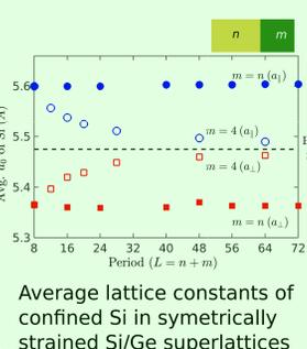
Average lattice constants of confined Si in symmetrically strained Si/Ge superlattices
